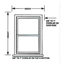
The Standard Window Size is (3'x5') 35"x60". This worksheet is based on this standard 3'x5' – most installed size window on homes and is usually located on all 4 sides and the 2<sup>nd</sup> story.
